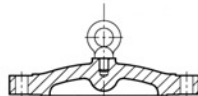
COVER & EYEBOLT ARRANGEMENT FOR VALVES 14" & ABOVE (CLASS 150), VALVES 10" & ABOVE (CLASS 300) & VALVES 4" & ABOVE (CLASS 600)
